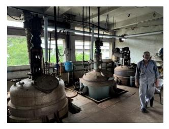
**Polymerization Reactor (SS Reactor)**
