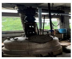
**Mixing Reactor (SS Reactor)**
